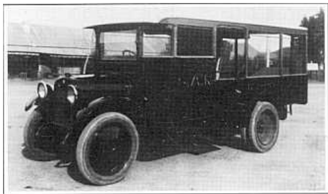
Early model, roofed dual-purpose vehicle. Passenger seat and partition just visible. Wire netting and roll-down blinds offered some protection.*
